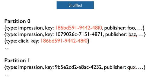
Figure 8: A shuffle operation ensures events to be joined at stored in the same Kafka partition.
