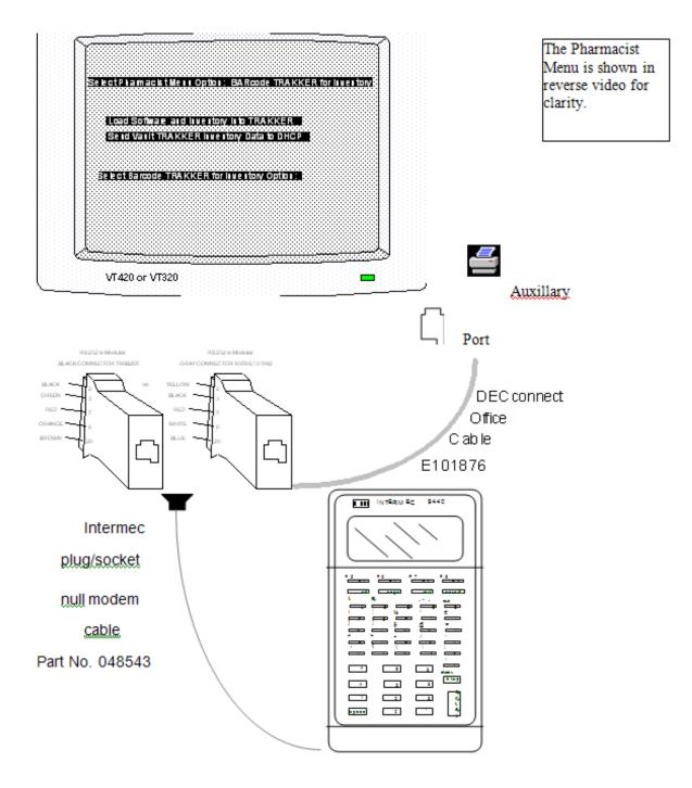
The PRINTER SET UP SCREEN of the VT-320 will allow configuration of the CRT for use with a TRAKKER. To get to this screen:
