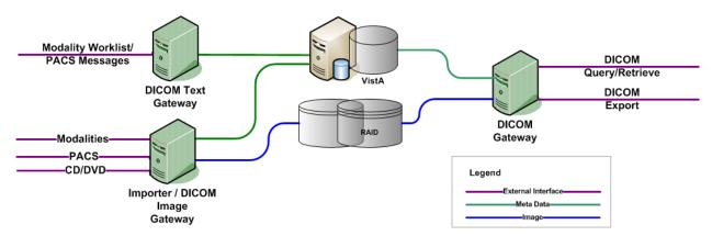
The software described in this document (the DICOM Gateway installation executable and the Java components) should be installed on all DICOM Gateways. Depending on the purpose of the gateway, several different configuration options can be used: Text Gateway, an Image Gateway, a Routing Processor, or any combination thereof. In addition, you can configure a Legacy Image Gateway to be a DICOM Importer. You can also enable the DICOM Query/Retrieve application server on a gateway.
