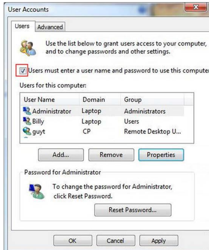
Figure 26 - User must enter a user name and password to use this computer option
