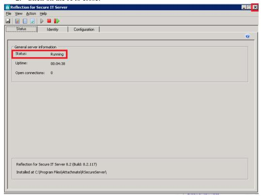
Note: This step is required to force Reflection for Secure IT Server to load the configuration file. If the server has a Status of "Running" then the configuration file has been loaded.
