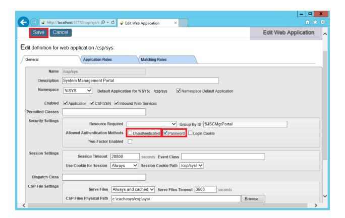
9. Check the Password box and then uncheck the Unauthenticated box. Click Save.
