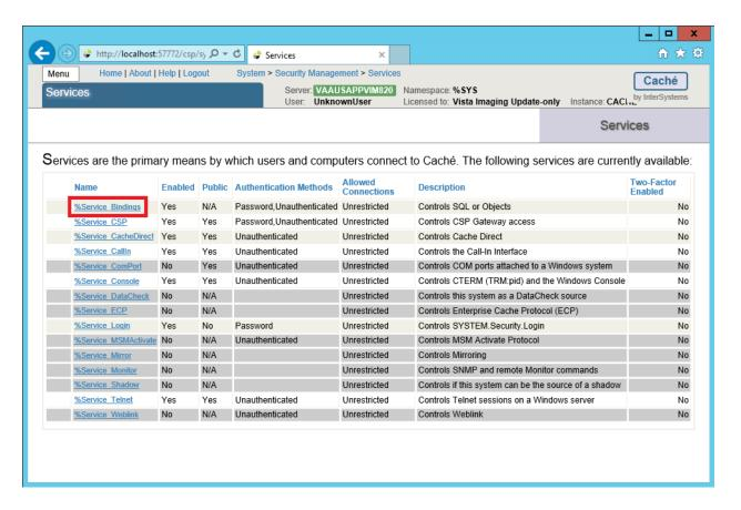
3. On the Services page, select **%Service\_Bindings** from the Name column to edit. This displays the definition of service **%Service\_Bindings** so that the authentication method can be configured.
